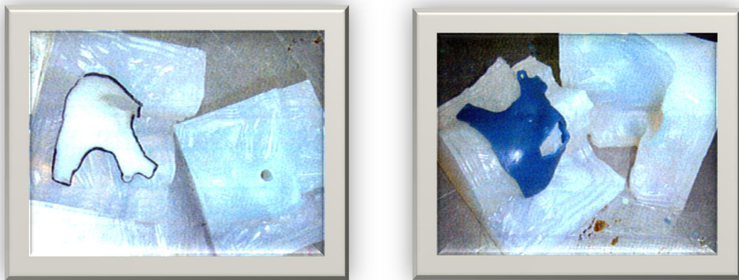
Figures 3 e 4: Stereolithography model (AM) used to manufacture the silicone mold and the silicone mold
