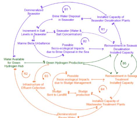
The second perspective compares upper and lower parts of the CLD. It considers the linear economy approach, featuring balancing loops B1 and B2, along with reinforcing loop R1. Subsequently, it considers the circular economy approach, incorporating balancing loops B3 and B4, and reinforcing loop R2. Lastly, balancing loop B5 highlights the selection preferences for water supply sources.
