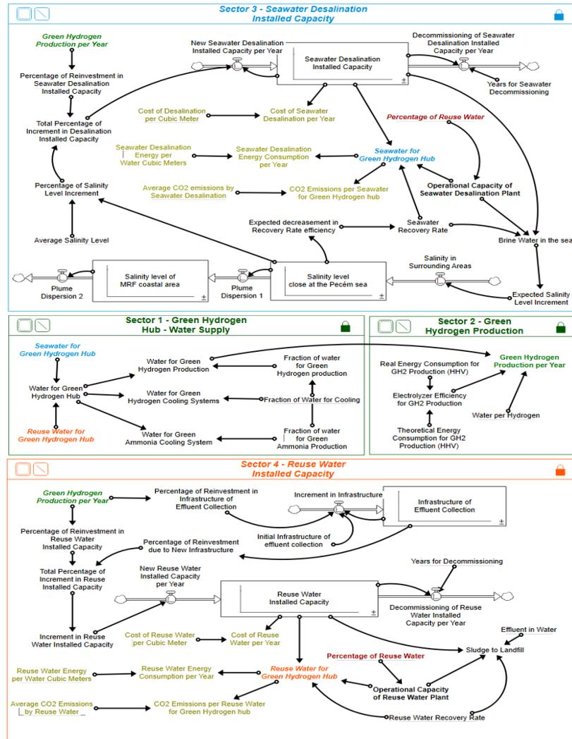
The SFD can be analysed by starting on sector 1 looking at the variable “*Water for GH hub*” (WGHH) as shown in equation 1, which depends on two other variables that come from both sectors 3 and 4. These are the “*Seawater for GH Hub*” (SWGHH) and the “*Reuse-water for GH Hub*” (RWGH). These major indicators can be calculated by the following equations:
